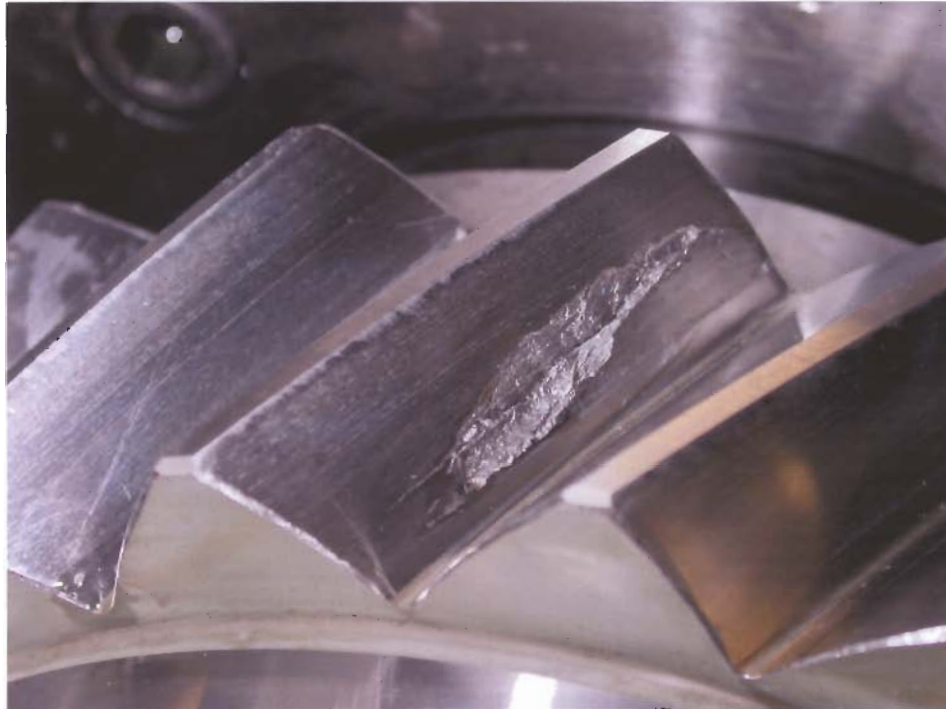
Figure 2.1: Edge cracking and secondary pitting damage on wheel flank of MEGAGEAR® G-B13210-3 after 5.77 \times 10^6 cycles (4500Nm, 100 cSt Mineral Oil + 4% Anglamol, 70°C, 3000rpm).
