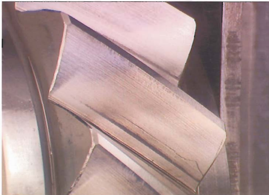
Figure 2.2: Edge cracking across face on wheel flank of MEGAGEAR® G-B13210-3 after 5.77 \times 10^6 cycles (4500Nm, 100 cSt Mineral Oil + 4% Anglamol, 70°C, 3000rpm).
