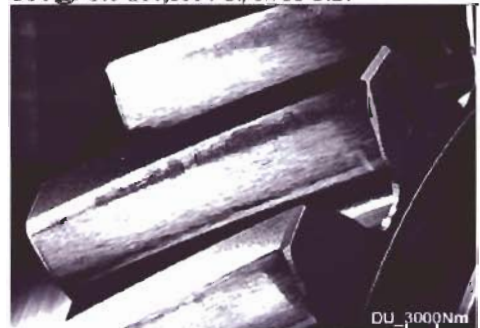
Standard gear 23 teeth, 4.233 NDP, 20° PA, 30° HA 1264 HP at 3000 RPM, 50 million load cycles SCS@PCR=231,000 PSI, 6.753 O.D.
